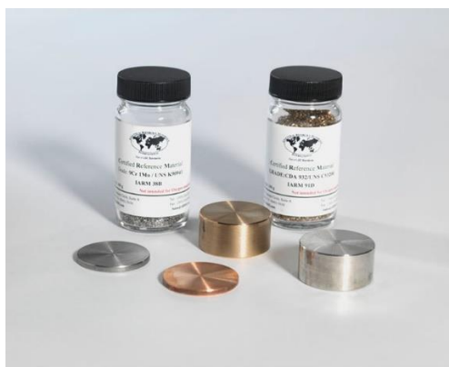
Calibration standards (Certified Reference Material- CRM) for XRF tests
